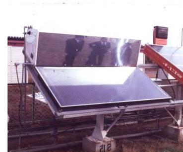
Fig.16 Solar water heater of gravity circulation type
