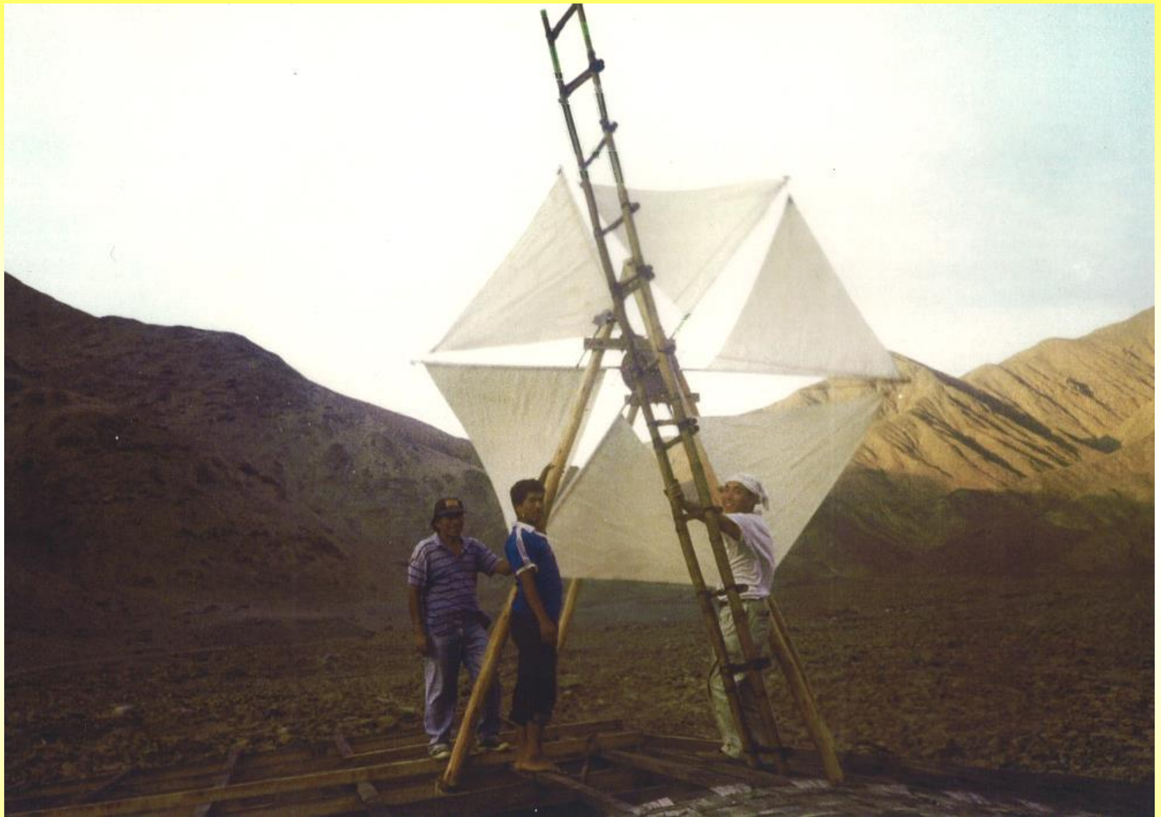
Sail-wing Windmill for water pumping in Peru by Dr. T. Dei
